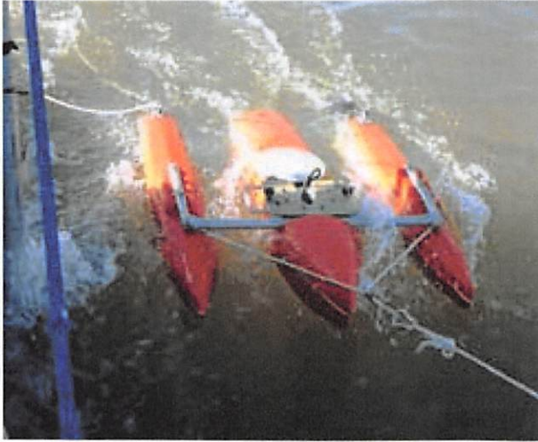
Figure 6. Teledyne RiverRay ADCP.
